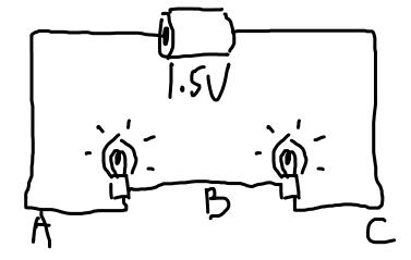
If wire resistance so Small we can reglect, then IC of change moving from A to B needs 0.75 J of work.
