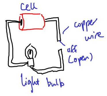
Electrons in copper start to flow when Switch is closed.
