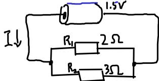
If I replace by a Single resistor R, what resistance would give the same current I as before?
