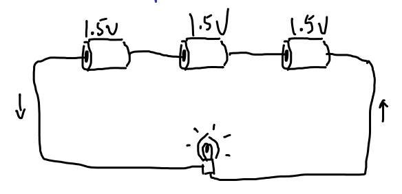
Each cell does 1.5J of work on 1C.
